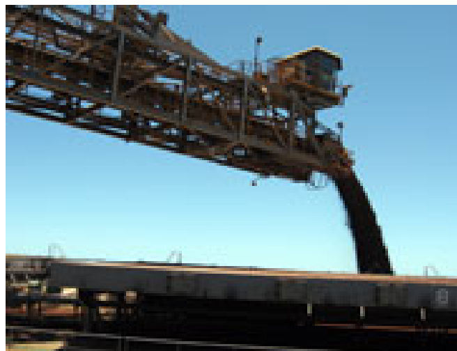
A Rio Tinto iron ore shiploader in operation in the Pilbara. Photo Chard Hargrave, CSIRO
